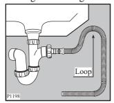
The drain hose may be extended to a maximum of 4 metres. An additional drain hose and joining piece is available from your local Service Force Centre.
